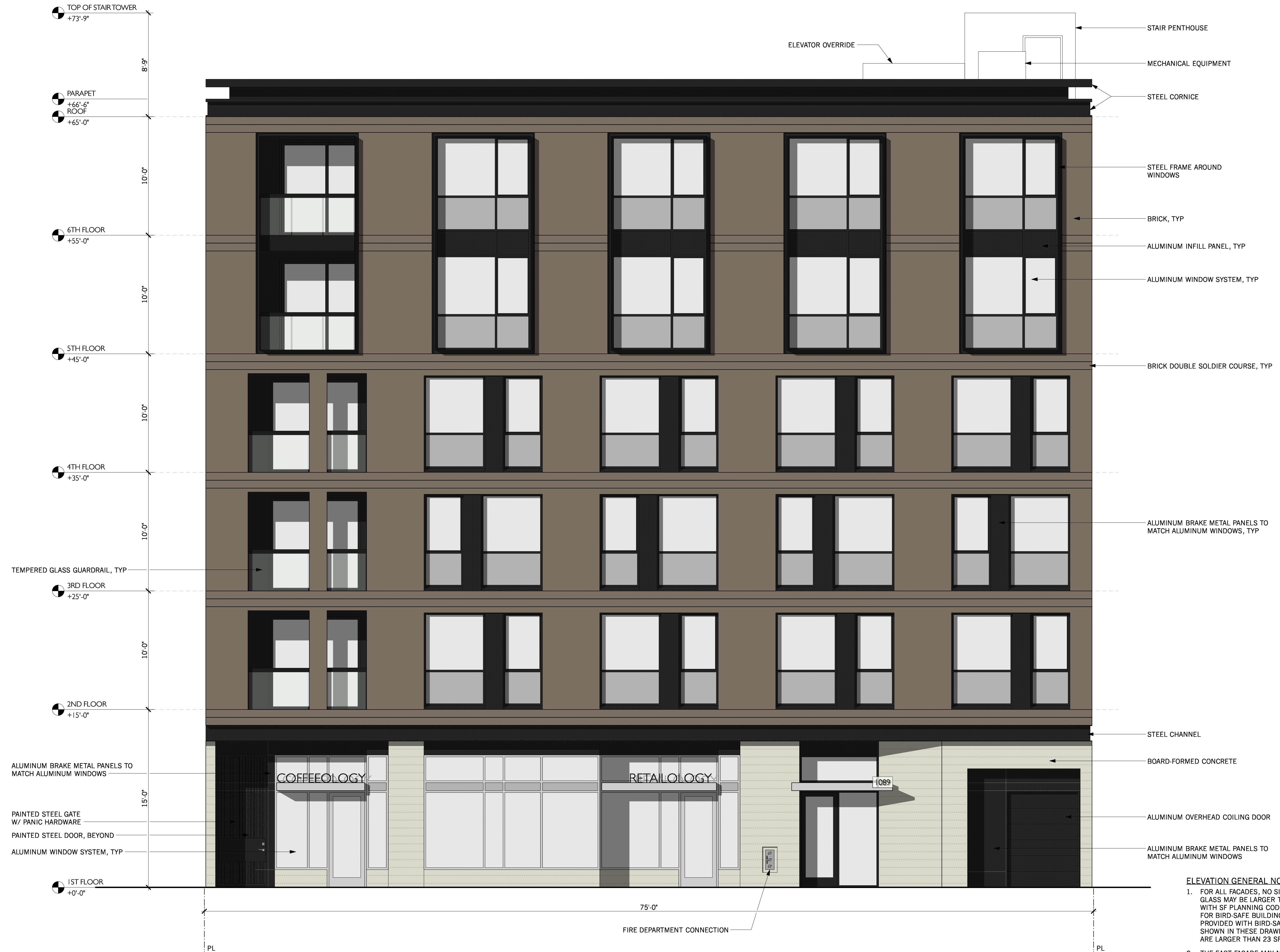
1 NORTH ELEVATION - FOLSOM STREET Scale: 1/4" = 1'-0"
