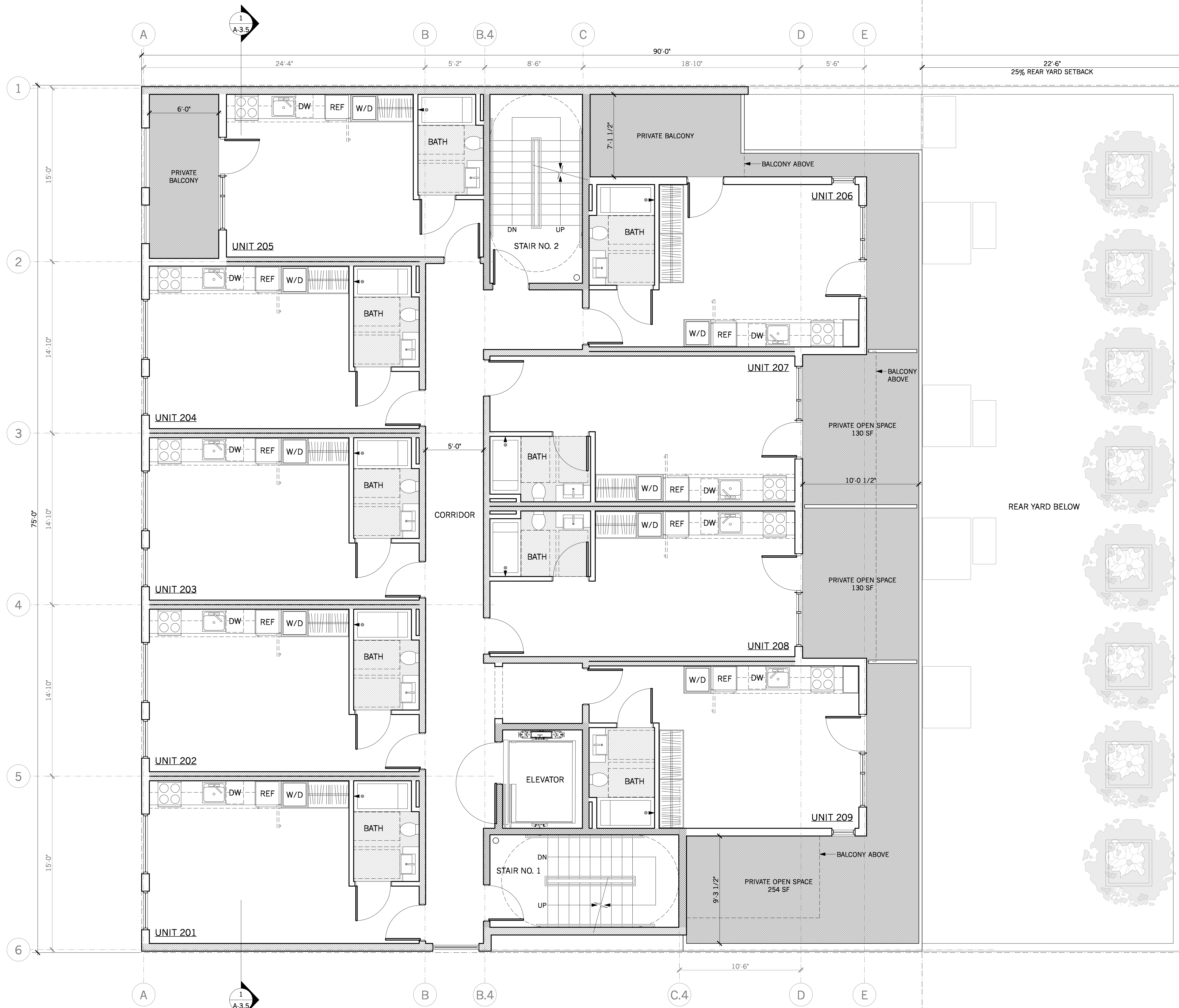
1 2ND FLOOR PLAN Scale: 1/4" = 1'-0"
